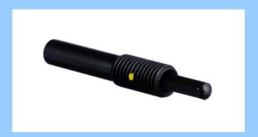
LONG TRAVEL HEX NOSE PLUNGERS are suitable for long-life, high-speed applications and can be easily adjusted, removed or inserted using a standard wrench from the plunger end.
